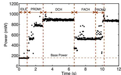
Fig. 1. Device Power at Different RRC States
