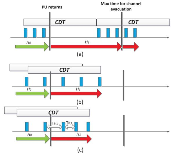
**Fig. 3:** Detection delay (indicated by the red arrows) with (a) forward, non-overlapping GD-SPRT; (b) backward, overlapping GD-SPRT; and (c) backward, overlapping GD-SPRT with short-term  $T_p$  adjustment
