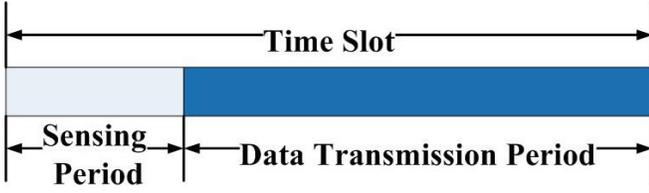
Fig. 1. The structure of a time slot.
